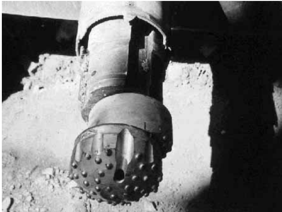
Figure 2 – Eccentric Hammer Inside the Casing
